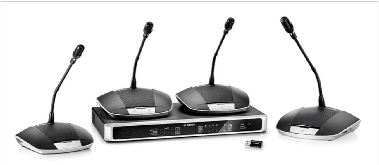
**Control unit** is the main device of VCS. You can connect to an Ethernet network, control the microphone settings and the progress of the conference with the help of this unit.
